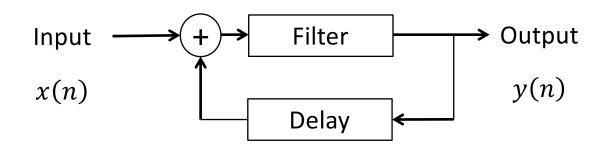
LTI digital filters allow to use the past outputs as input
