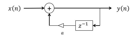
– When *a* is slightly less than 1, it is called "Leaky Integrator"
